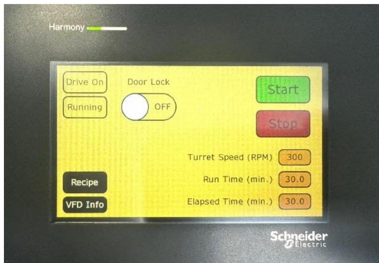
Once the machine comes to a full stop, select the **Door Lock** button to unlock the door.
