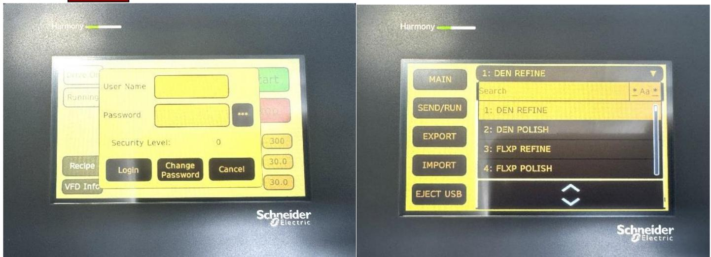
To Update software, download update to the USB Stick, insert it into the slot then select "Update". *We recommend backing up original data before updating.* The unit will update itself and reboot with the updated software. Ensure all the original recipes are still installed. Then select **Eject USB** to remove the USB stick. Click **Send/Run**, then click **Reset** to reset the "Fault" button. System is now ready.
