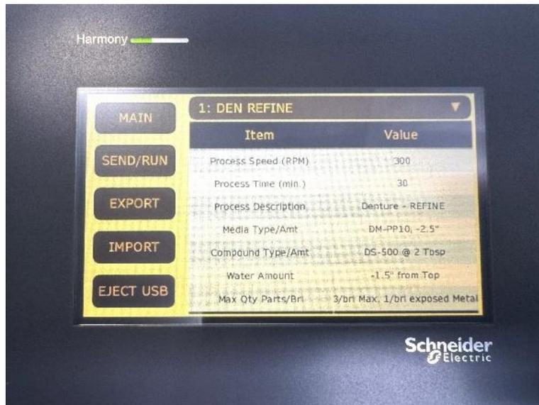
Click **IMPORT**, input login and password (default login is **Tech**, password is **autofinish**), press enter, then login. (The system will log out after five minutes) Select the "Import" button to import the data from the USB stick. Note that all the data in the HMI will be overwritten with new data. We recommend backing up original data. When done, select the **Eject USB** button to safely remove the USB stick
