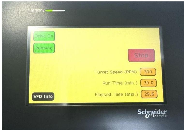
To view real time details on the speed, and power consumption select **VFD Info**
